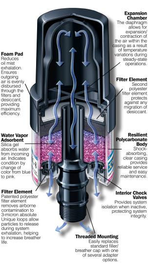
unit, multiple 3-micron polyester filter elements remove solid particulate and the color-indicating silica gel extracts moisture.
